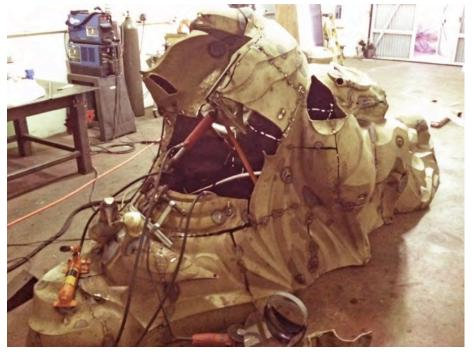
• Parts of the surface are "chased", or smoothed and somewhat polished, before the projecting parts are attached so that all areas can be easily accessed.
