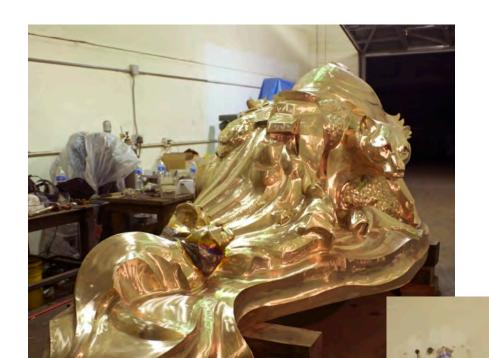
• When the last of the welds is chased out, the piece is ready to deliver for patina.
