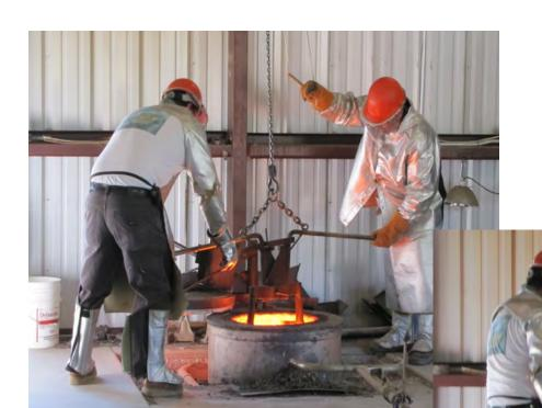
• When the proper temperature is reached, the glowing hot crucible is removed from the furnace and carried to the sand box full of molds for pouring.
