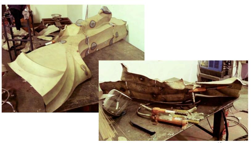
• Ill-fitting pieces are forced into shape and welded into place.
