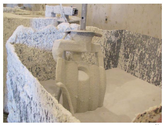
• This process was repeated many times to build up the shell mold on all sides of the panels (and both inside and outside of hollow pieces). Each panel was air dried between each coat of slurry and sand and after the final coat.
