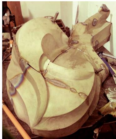
• Once the panels are tacked in place, the welds are completed and feathered out to create a level surface when finished.
