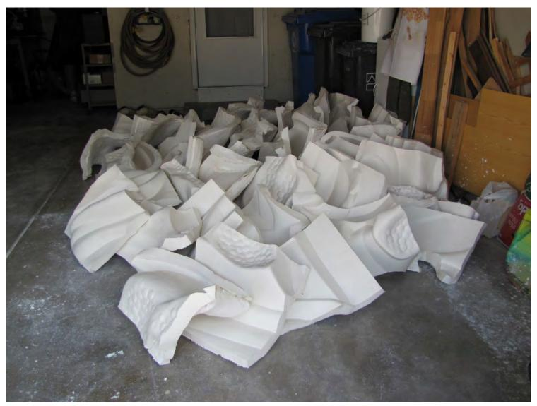
\* Each mold section was used to create a wax panel for casting in bronze.
