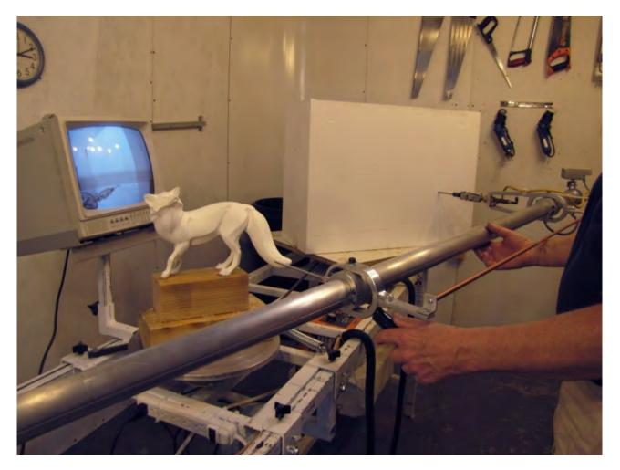
• The burner point carves out the enlarged duplicate of the model, slightly smaller than the desired end result to allow room for an added layer of clay.
