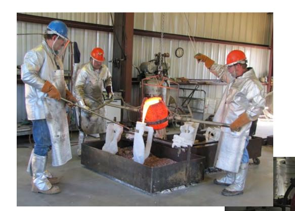
• Each mold is carefully filled with molten bronze until the crucible is empty.
