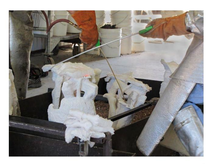
• Once the bronze has cooled, the shell mold is broken off and the cast bronze cleaned to reveal the results of this complex process.
