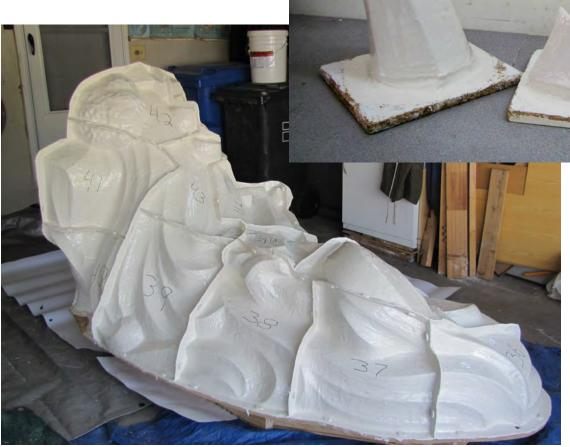
• Once the rubber had set up, individual batches of plaster were mixed to be applied as backing, or "mother mold," to support the rubber panels when removed from the clay.
