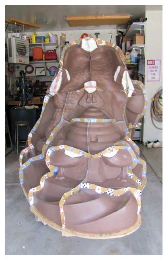
• A rubber compound was carefully measured and thoroughly mixed and every batch of rubber tested by heating and drying it quickly to be sure that it has been mixed properly to set up correctly.
