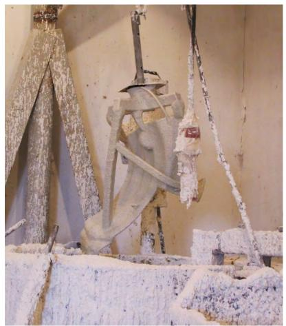
• After the slurry, each panel was dipped into a vat of silica sand which is injected with air, enabling the panel to be easily immersed and coated with the sand.
